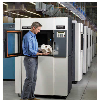
FIGURE 2. Stratasy's Fortus 360mc 3-D production system. (Source: Stratasy Inc.)
