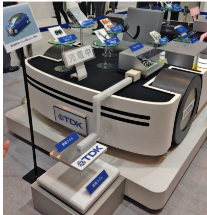
FIGURE 7. The TDK concept magnetic resonance system. (Photo Courtesy of O & S Services Inc.)
